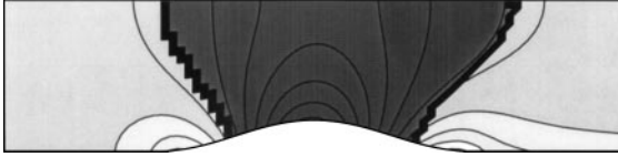
FIG. 6. Channel with bump. Logarithm of the Mach number (min = 7.668 \cdot 10^{-3} , max = 0.4136, 80 isolines in logarithmic scale). Note the sharp discontinuity along the phase transition line.
